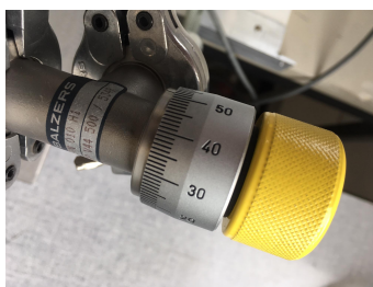
Figure 1.11: Important: A needle valve must not be tightened like a water tap! As soon as you feel little resistance while turning and the pressure on the digital manometer remains stable, the valve is closed. Further tightening can damage the needle valve.
