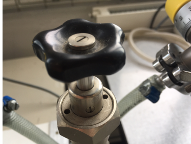
Figure 1.9: The black valve used to vent the vacuum pump. Always vent the pump immediately after use to avoid oil being sucked in.
