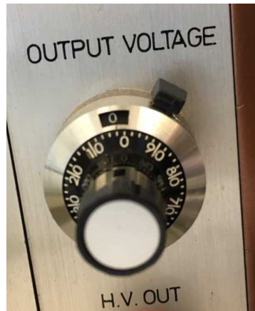
Figure 1.10: This rotary switch is used to set the high voltage for the semiconductor detector. To set 100 V, the top display must show 1 and the dial 0. For 130 V, the top must show 1 and the dial 30. When switching on or off, both should be set to 0 as shown.
