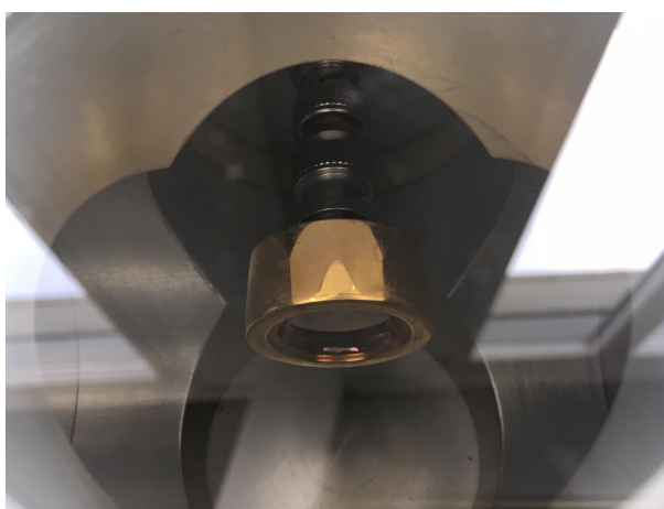
Figure 1.7: The silicon semiconductor detector has a circular entrance window. The ^{241}\text{Am} source, which emits alpha particles, is positioned opposite the detector.
