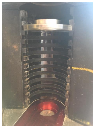
Figure 1.10: Place the transparent sample holder containing the filled dish in an upper position inside the measurement chamber. During the measurement, the lead door of the chamber must remain closed at all times.
