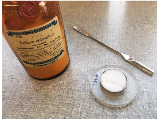
Figure 1.9: Potassium chloride is filled into the inactive sample dish up to the brim. Use a spatula for this purpose. Wear gloves and handle carefully to avoid spilling. The sample dish is then placed in a transparent sample holder.
