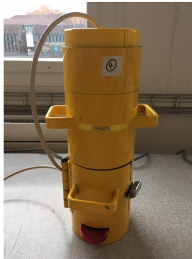
Figure 1.5: For determining the half-life of ^{40}\text{K} , a PHILIPS counting tube is used. It is encased in lead. At the lower section is the measurement chamber, into which the samples can be inserted.
