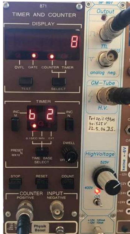
Figure 1.8: The brown module on the left is the counter; the silver one on the right is the high-voltage supply for the counting tube. To switch on the high voltage, turn the main switch on the far right to ON, and then switch the high voltage to ON at the bottom of the silver module. A value of 580 V should be set. The output signal is to be connected to the counter. The dead time of the counting tube is approximately 190 \mu\text{s} .
